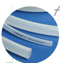
dvantaFlex TPE (thermoplastic elastomer) tubing addresses the need for a flexible, translucent, sterilizable, moldable, heat sealable, and weldable biopharmaceutical tubing for fluid processing. AdvantaFlex maintains its physical properties following sterilization processes, resists kinking, remains translucent for visible product flow, and does not become gummy. Additionally, the unique properties of AdvantaFlex help it outperform similar tubing in peristaltic pumps.
