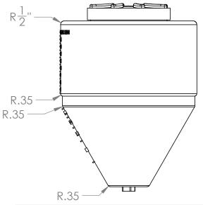
DIMENSIONS ARE IN INCHES NAME DATE TOLERANCE: ± 1/4" CDH 7/18/16 DRAWN MATERIAL LLDPE - FDA resin APPROVED CAPACITY **REVISIONS** ZAK 7/20/17 15 Gallon
