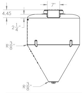
DIMENSIONS ARE IN INCHES NAME DATE TOLERANCE: ± 1/4" CDH 7/18/16 DRAWN MATERIAL LLDPE - FDA resin APPROVED CAPACITY **REVISIONS** 7/21/17 ZAK 65 Gallon
