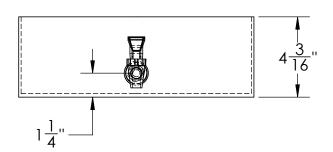
DIMENSIONS ARE IN INCHES NAME DATE TOLERANCE: ± 1/4" JMP 6/20/19 DRAWN MATERIAL WELDED HDPE APPROVED CAPACITY COMMENTS: 1.8 Gal.
