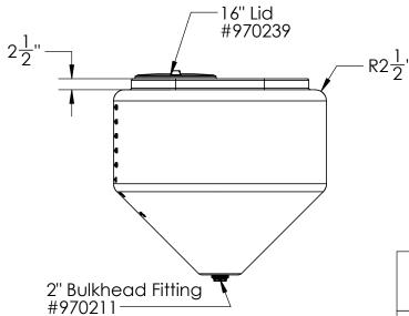
200 Gallon Cone Bottom Tank w/ 16" Lid & 2" Bulkhead Fitting
