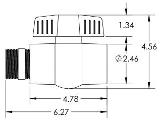
1.5" Valve Kit: Ball Valve & Pipe Nipple
