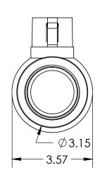
2" Valve Kit: Ball Valve & Pipe Nipple
