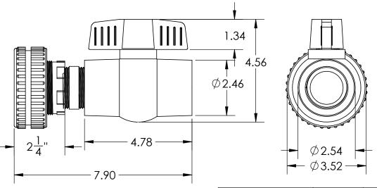
1.5" Valve Kit: Ball Valve, Pipe Nipple & Fitting
