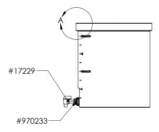
Standard Weight Polyethylene Storage Tank w/ External Flange w/ Spigot
