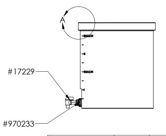
Heavy Weight Polyethylene Storage Tank w/ External Flange w/ Spigot
