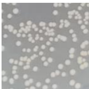
Standard silicone, after 24h. Bacteria growth.
