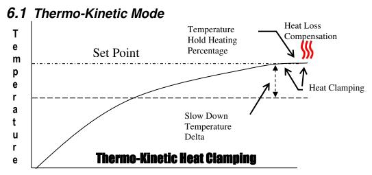
Setup settings "Slow Down Temperature Delta" and "Hold Percentage" configure Thermo-Kinetic Mode. The default settings are 10 degrees C Slow Down Delta and 10% power Hold Heating percentage.
