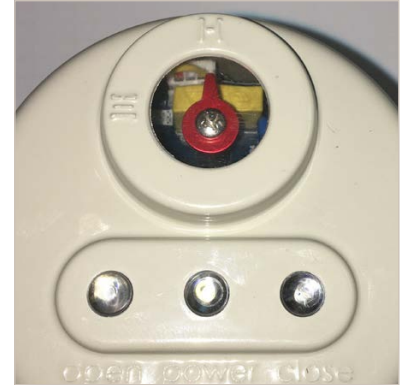
The actuator has a red pointer type position indicator. Pointing at the “] – [” means the actuator is fully CW. Pointing at the “] | [” means it is fully CCW.
