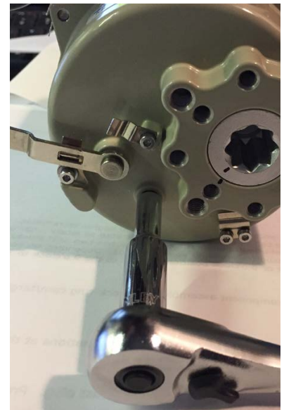
The 5mm hex manual override allows a user to position the valve or damper with or without power. See Declutch Lever for Manual Override section for details.
