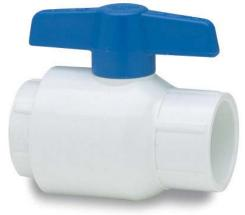
A high quality, economical quarter-turn shutoff valve designed for irrigation, pool and spa, and general purpose applications. IPS sizes 1/2" - 2" available in PVC White, PVC Gray or CPVC with socket or threaded end connectors. Sizes 3" - 4" available in PVC White with socket or threaded end connectors. 6" size available in PVC White with socket end connectors and high-efficiency lever style handle for easier operation.
