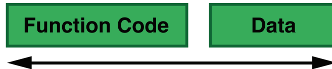
Figure 1: MODBUS Protocol Data Unit
