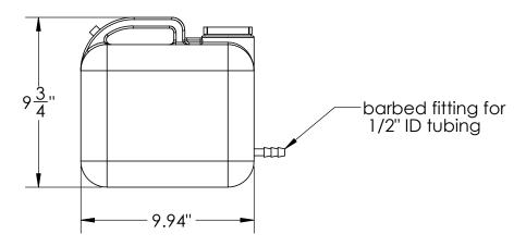
Fort-Pak Modified by Tamco with a barbed fitting for 1/2" ID tubing #76887
